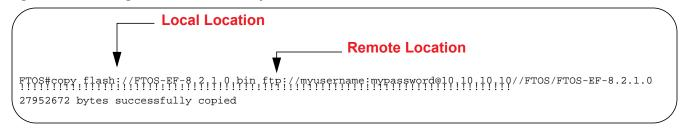
Figure 3-5 shows an example of using the **copy** command to import a file to the Dell Force10 system from an FTP server.
